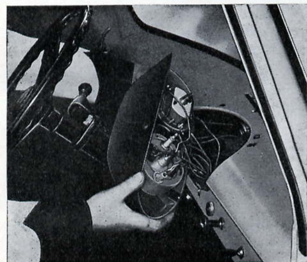
Fig. T.7. View showing instrument cluster panel detached and cable disconnected from speedometer
