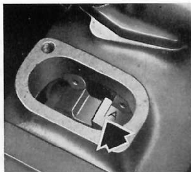
Fig. D.8. DPA pump timing. The flange marks must be aligned as shown on the left. On the right, the scribed line marked 'A' on the pump rotor must be aligned with the squared end of the preset timing circlip
