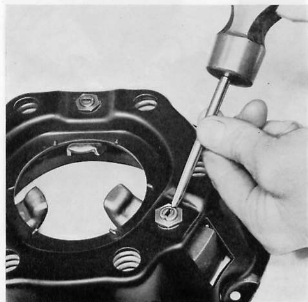
Fig. E.11. Locking an eye bolt nut by staking the nut collar into each end of the bolt slot
