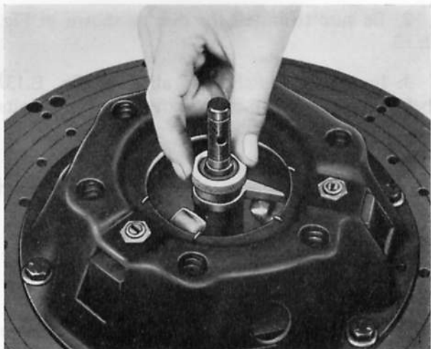
Fig. E.10. Checking the height of a release lever. Height adjustment is made by rotating the eye bolt nuts
