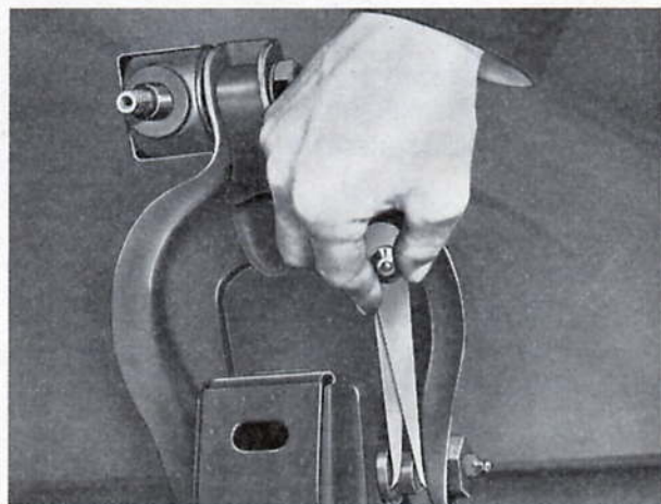
Fig. K.30. Checking the location of the upper arm in relation to the crossmember. The arm is raised from the horizontal position for the purpose of illustration
