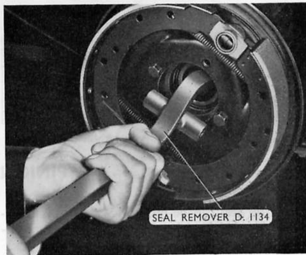
Fig. J.7. Removing an axle shaft oil seal
