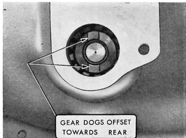
Fig. A.27. Installed position of oil pump drive gear offset dogs
