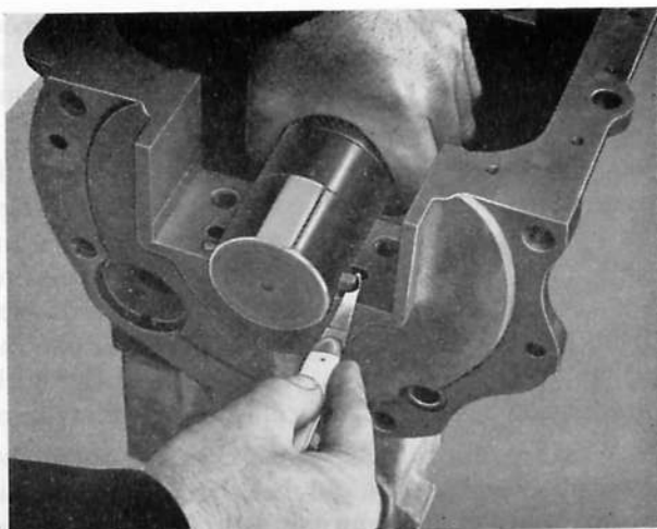
Fig. A.57. Cutting the oil seal ends flush with the bearing joint face. The seal must then be smeared liberally with the recommended lubricant
