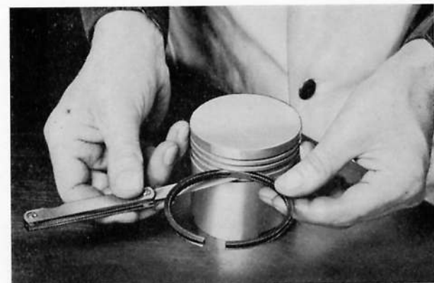
Fig. A.38. Checking piston ring side clearance in piston groove
