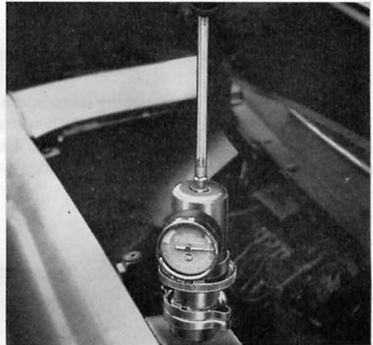
Fig. C.5. Pressure testing the radiator filler cap and the seating in the radiator filler neck
