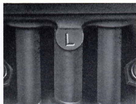
Fig. A.34. Cylinder head identification. Letters 'L' and 'H' indicate respectively a low and high compression ratio head
