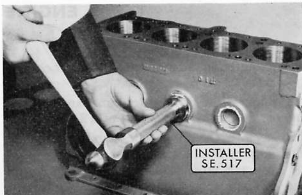
Fig. A.48. Installing a small cup plug, using Drift SE.517. Use Drift SE.123 when installing the larger cup plugs
