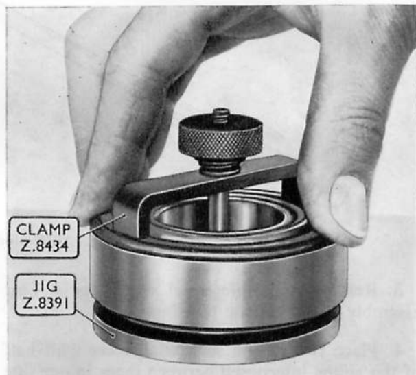
Fig. J.24. Settling the pinion bearing on the measuring jig
