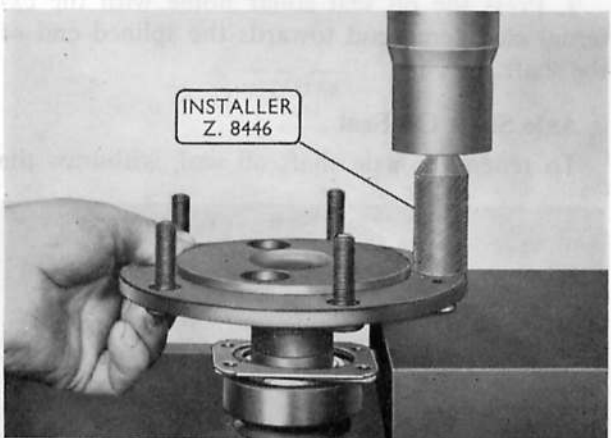
Fig. J.9. Pressing home a new wheel bolt
