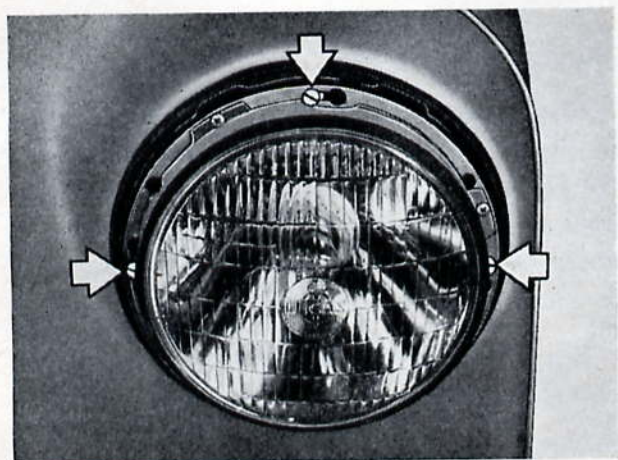
Fig. S.3. The arrows indicate the lamp beam trim screws
