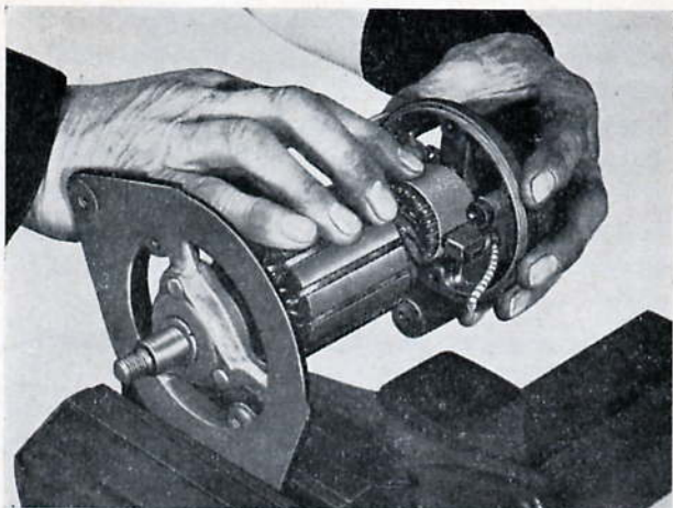
Fig. P.22. Bedding-in new brushes with fine grade glass paper wound round the commutator, which is then rotated
