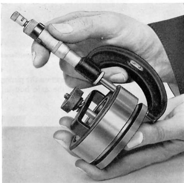
Fig. J.25. Measuring the overall dimension of the pinion rear bearing and jig plate
