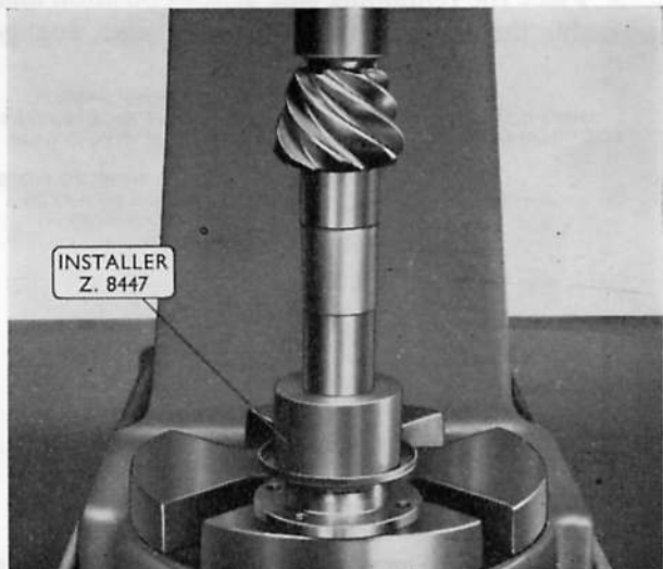
Fig. J.18. Pressing a new dust shield on the universal joint coupling flange
