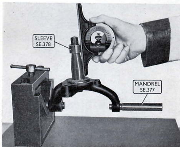
Fig. K.17. Checking the steering knuckle for distortion
