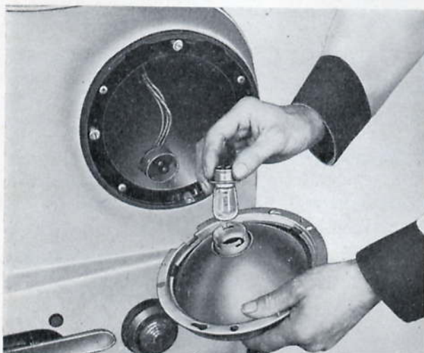
Fig. S.5. Installing the bulb in a pre-focus head lamp (not Unified European type). A slot in the bulb flange locates in a projection on the light unit
