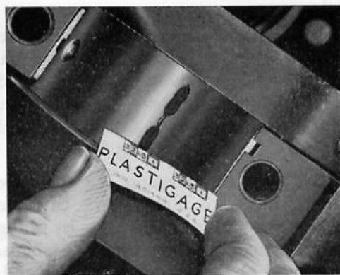
Fig. A.52. Use Plastigage for checking journal to bearing clearance. Left: Plastigage placed on journal. Right: Measuring width of compressed Plastigage; in this example the clearance is .0015 in.
