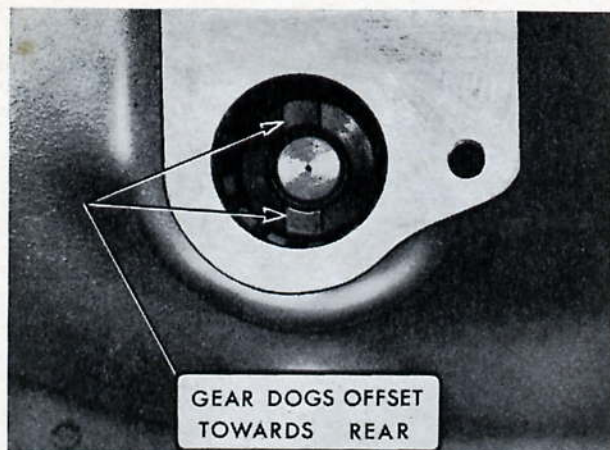
Fig. R.7. Location of oil pump drive gear dogs when installing the distributor. The dogs are at right-angles to the camshaft and offset as shown
