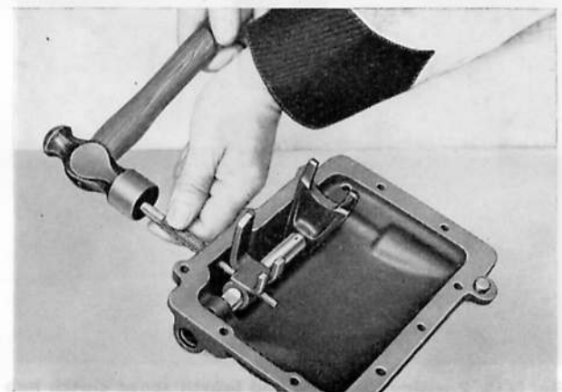
Fig. G.17. Driving out the reverse shift fork retaining pin
