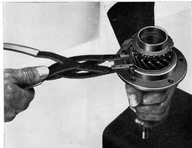
Fig. G.13. Releasing the main drive pinion and bearing from the front cover
