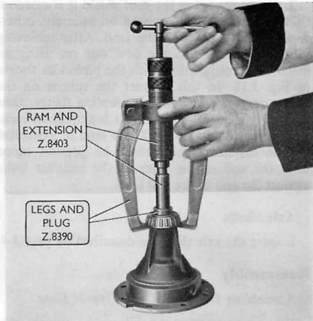
Fig. J.17. Removing a differential side bearing
