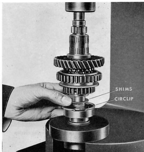
Fig. G.35. Pressing the bearing on to the mainshaft
