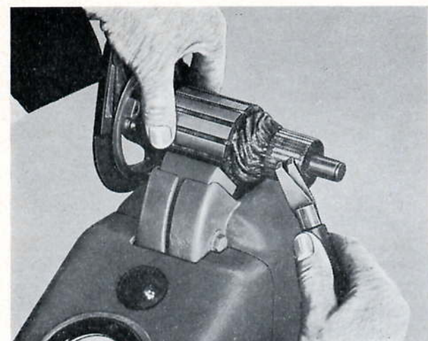
Fig. P.19. Testing armature windings for open circuits
