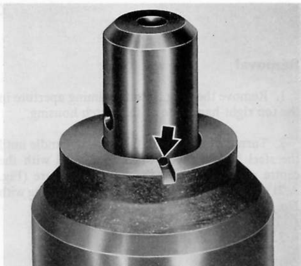
Fig. A.24. With the driving impeller pressed against the body, check that each oil metering hole in the shaft (arrowed) is fully uncovered when facing the slot
