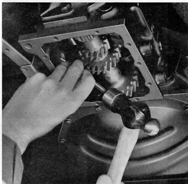
Fig. G.8. Driving out the striking lever shaft oil seal
