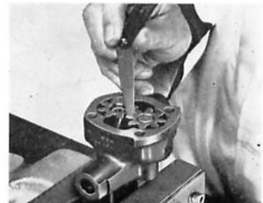
Fig. A.22. Checking oil pump impellers. From left to right—end clearance, radial clearance, and backlash
