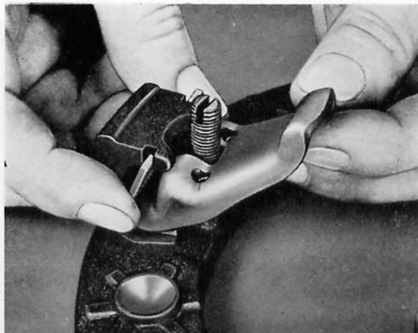
Fig. E.9. Assembling a release lever to the pressure plate. The strut must engage the grooves in the plate boss and the recess in the lever
