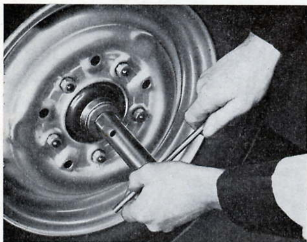
Fig. K.8. Initial tightening of the front hub nut, using a tube wrench and bar
