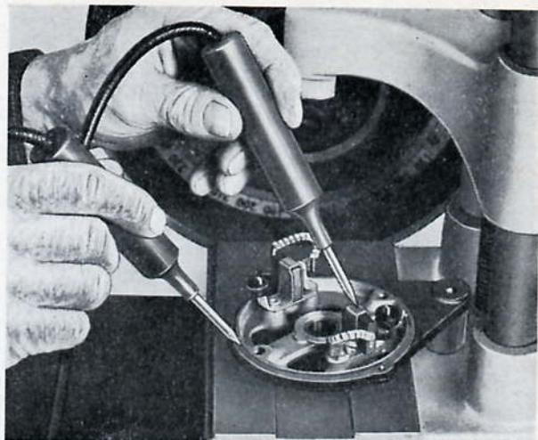
Fig. P.24. Testing brush holder insulation
