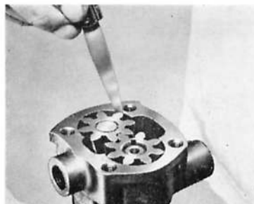
Fig. A.22. Checking oil pump impellers. From left to right—end clearance, radial clearance, and backlash
