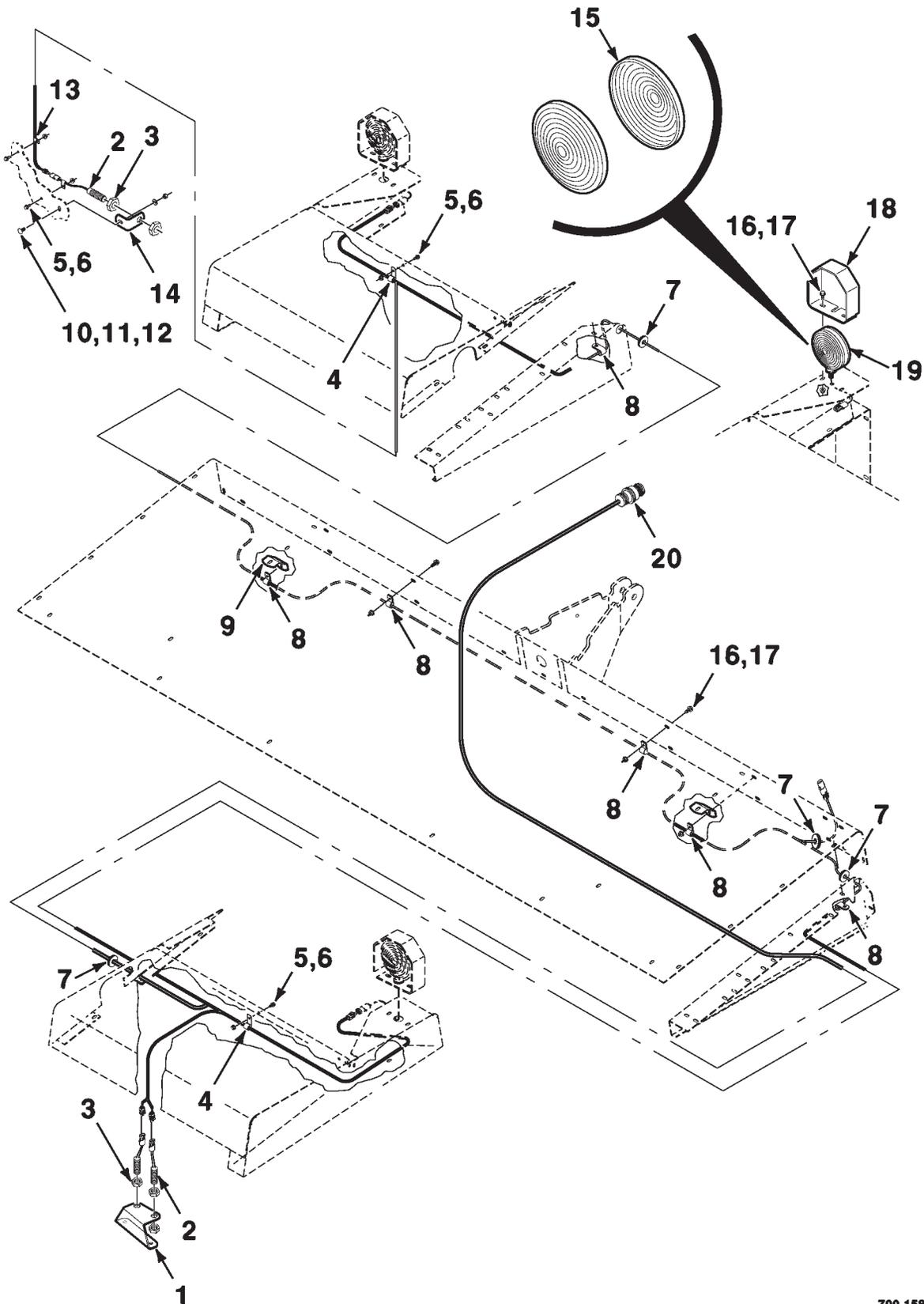
**DKHB ROTARY HEADER****83****ELECTRICAL****ELECTRICAL HARNESS AND FLASHER (15 FOOT)**
