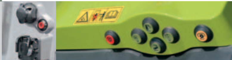
External controls for front and rear PTO
