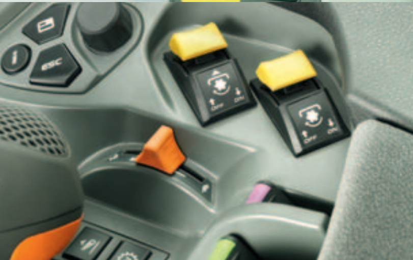
External controls for front and rear PTO
