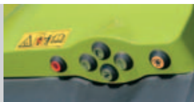
External controls for the rear linkage, PTO and one freely selectable spool valve
