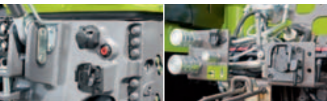
ISOBUS connections at the front and rear
