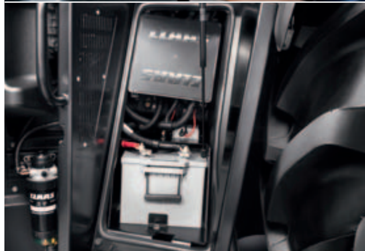
The fuel prefilter is conveniently located by the steps to the cab.
