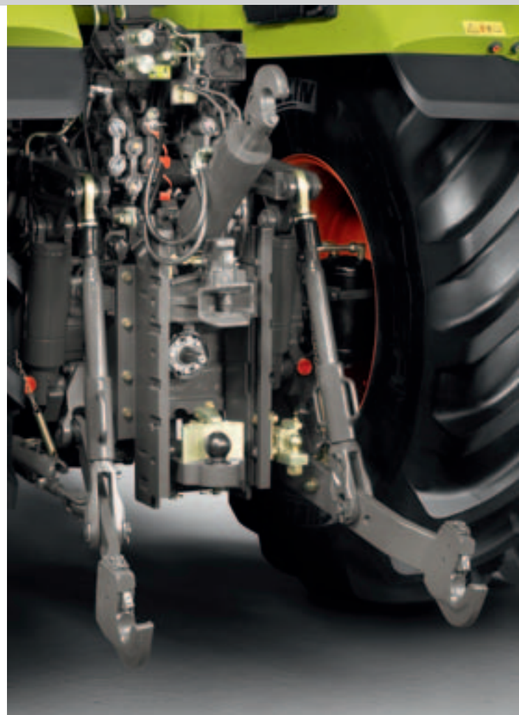
External controls for the rear linkage, PTO and one freely selectable spool valve
