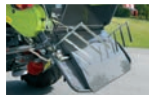
Swath former on the deflector
