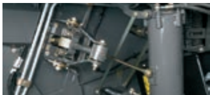
3D-cleaning system hydraulic control unit
