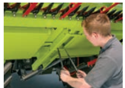
Adjusting the table length of the CERIO 930 and 770
