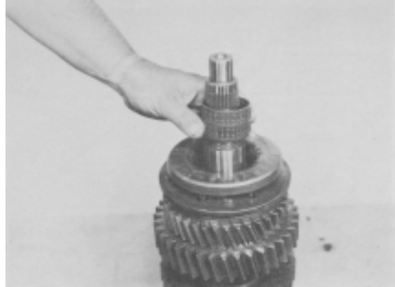
Figure 52 - Install 3rd speed gear roller bearing.
