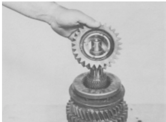
Figure 53 - Position 3rd gear on bearing with clutching teeth down.
