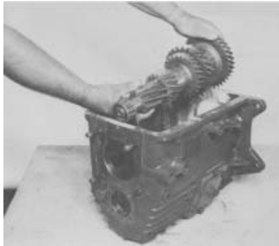
Figure 12 - Remove countershaft assembly.
