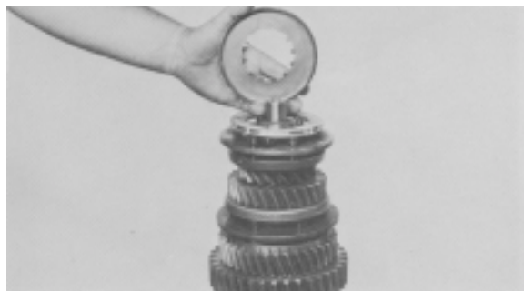
Figure 18 - Remove 5th-Speed synchronizer cup.
