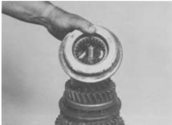
Figure 20 - Remove 4th & 5th speed synchronizer assembly/
