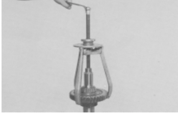
Figure 37 - Remove Reverse speed gear and rear bearing from mainshaft.
