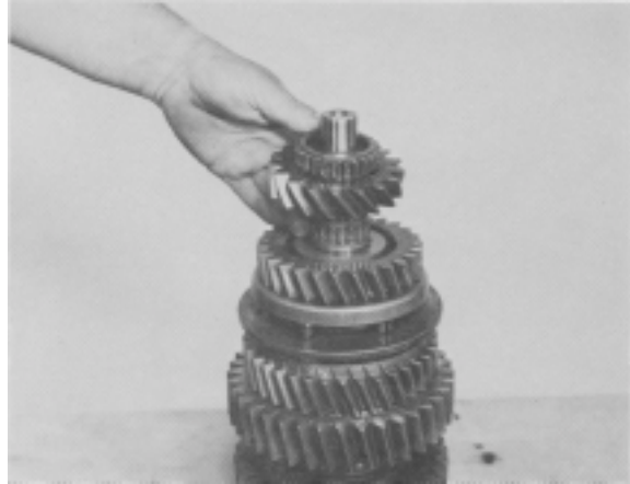
Figure 22 - Remove 4th speed gear.
