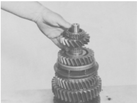
Figure 57 -Position 4th gear on bearing with clutching teeth up.
