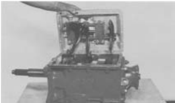
Figure 2 - Remove control cover assembly.
