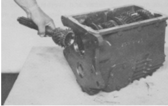
Figure 7 - Remove main drive gear and bearing assembly.
