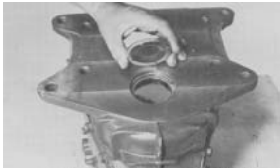
Figure 89 - If the transmission case or countershaft front taper bearing cup was replaced, install bearing cup locating ring. From inside of case, install bearing cup. Coat outer diameter of bore plug with Loctite 510 and install bore plug in case.
