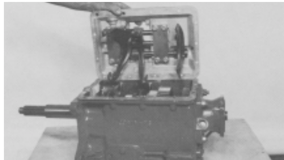
Figure 106 - Locate control cover gasket on transmission case. With transmission in neutral, position control cover over gears aligning shift forks in shift cover with gear shift hubs. If control cover is in neutral and transmission is in neutral, transmission drive gear should turn without output shaft turning.
