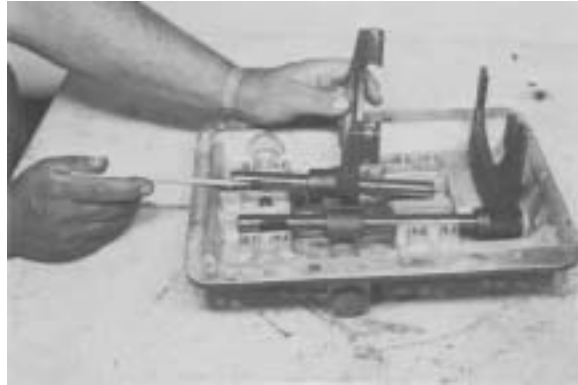
Figure 81 - Install interlock cross pin in 2nd & 3rd shift rail. Position 2nd & 3rd shift rail and fork assembly in rail groove over mesh lock ball and spring. Make certain cross pin is in position in rail. (See Figure 78-A).
