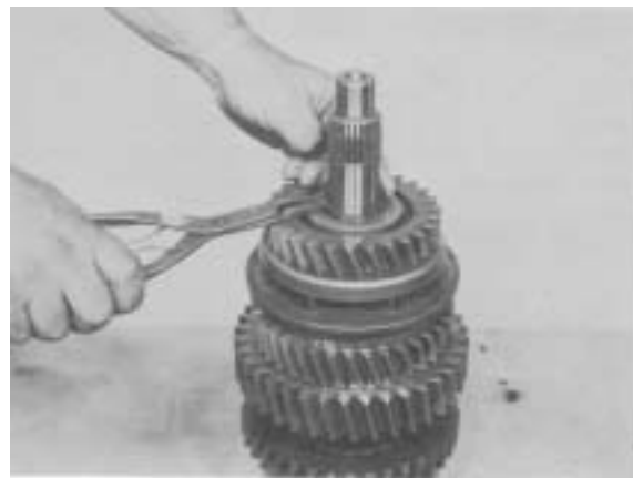
Figure 24 - Remove 3rd gear locating washer retaining ring.
