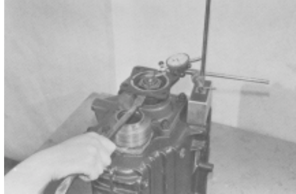
Figure 105 - Place transmission in vertical position, with main drive gear pointing down. Install transmission output flange and nut. Roll main drive gear and mainshaft to seat front and rear taper bearings. Position a dial indicator as shown. Pry on output flange to get mainshaft and play. End play must be between .002 - .008. Add shims for more end play or remove shims for less end play.
