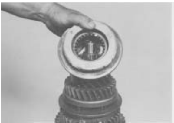
Figure 59 - Position 4th speed synchronizer cup and 4th & 5th synchronizer on shift hub sleeve.
