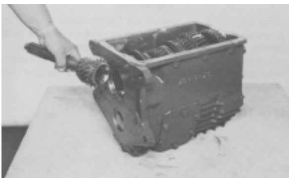
Figure 98 - With main drive gear needle rollers in place and greased, position main drive gear in housing bore. Align clutching teeth on main drive gear with teeth in 5th speed synchronizer cup.
