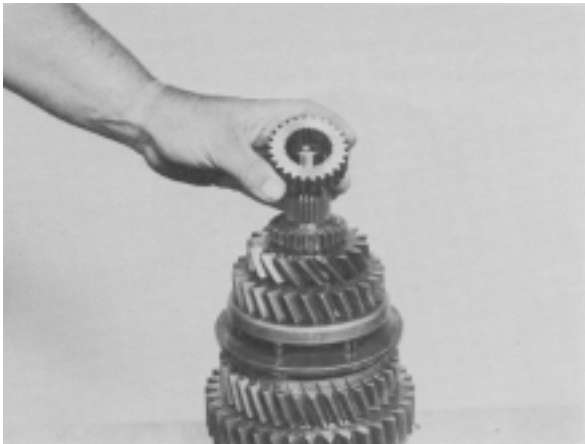
Figure 21 - Remove the 4th & 5th shift hub sleeve.
