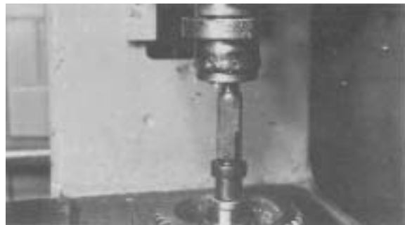
Figure 17 - With drive gear, snap ring out of groove, press countershaft drive gear and front taper bearing inner race from shaft. Press 4th gear from shaft. Remove gear keys from countershaft. 3rd speed and 2nd speed gears are splined on the countershaft and may be pressed from shaft, if replacement is necessary.
