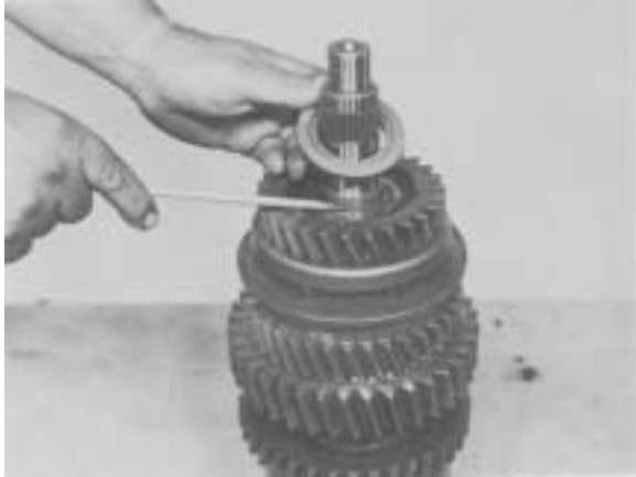
Figure 25 - Remove washer and lock ball.
