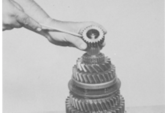
Figure 58 - Install 4th & 5th shift hub sleeve. NOTE: machine ground surface must be up.
