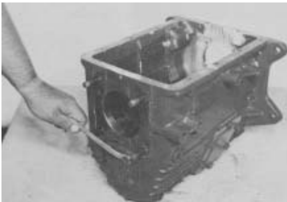
Figure 9 -Remove countershaft bearing cap bolts.
