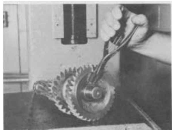
Figure 66 - Install drive gear retaining ring. NOTE: Make sure retaining ring is in full position in ring groove.
