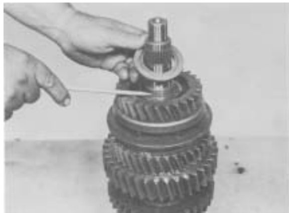
Figure 54 - Position 3rd gear locating washer lock ball in mainshaft. Install locating washer on shaft with notch in washer on lock ball.
