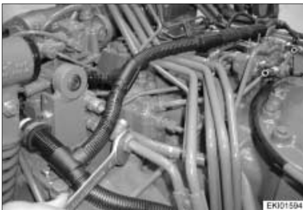
Fit lift cylinder pressure pipe.
