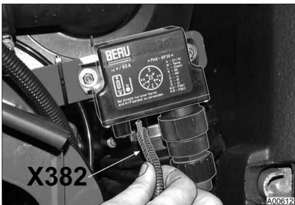
At bottom of A012 - ECU, cold-start aid X382 = Terminal for pin 30 (B+)
