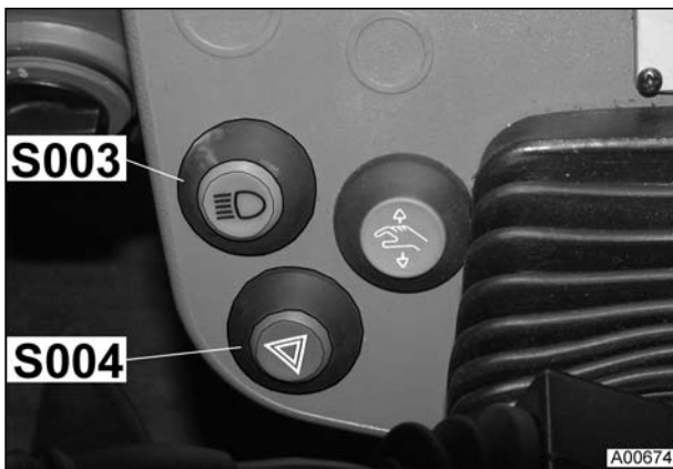
S003 = Switch, headlights S004 = Switch, hazard warning lights On left of instrument panel by steering wheel
