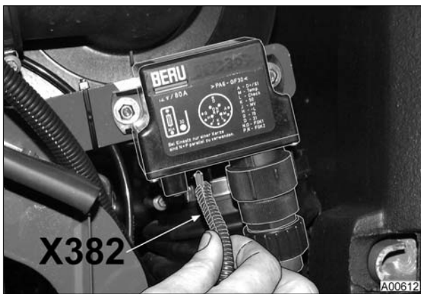
At bottom of e-box of cold-start aid A012 X382 = terminal for contact 30
