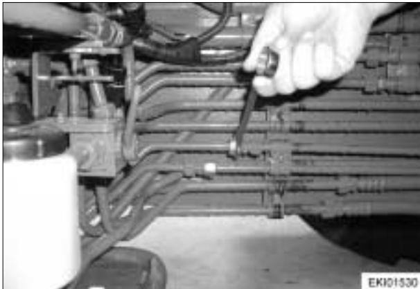
Fit hydraulic lines to front PTO.
