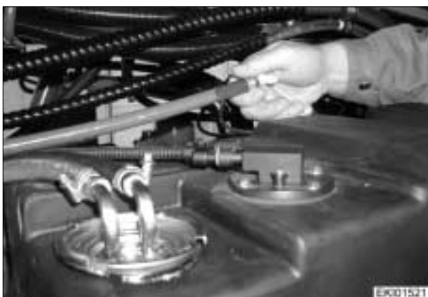
Fit tank venting tube.
