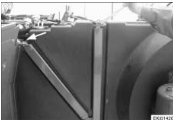
Fit clamp, brace and bracket (arrowed).
