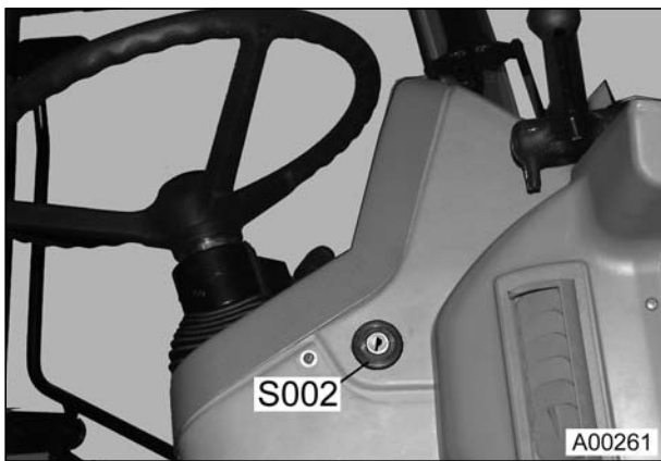
S002 = Switch, ignition On right of steering column
