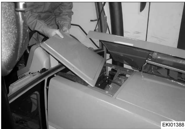
Raise side sections and remove cover panel.
