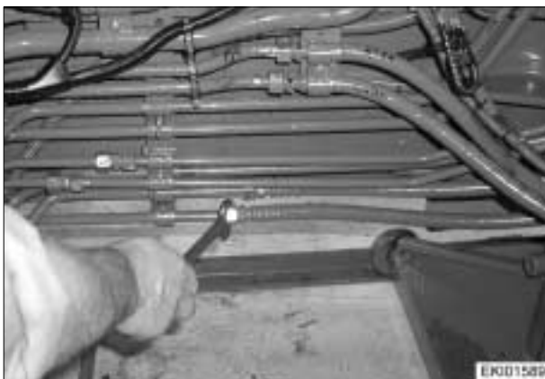
Fit hydraulic lines to front-axle suspension and fit clip.
