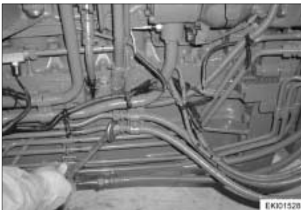
Fit hydraulic lines to steering cylinder.
