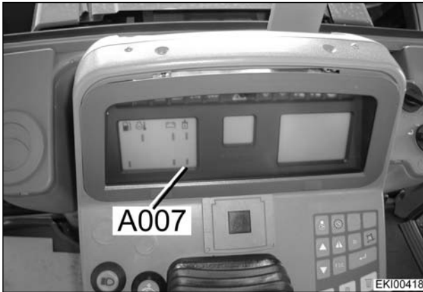
A007 = Display unit At top of steering column
