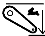
Fig. 5 Key on membrane keypad with "Active" LED on control console Rapid lowering system only available on rear power lift
