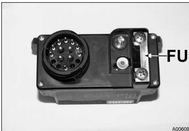
At bottom of e-box of cold-start aid A012 FU = 80 amp fuse
