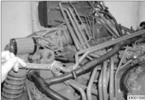
Fit both connecting lines of lift cylinders.
