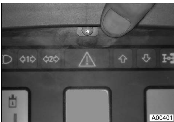
Dimmer control at top of instrument panel. Current and voltage will vary.
