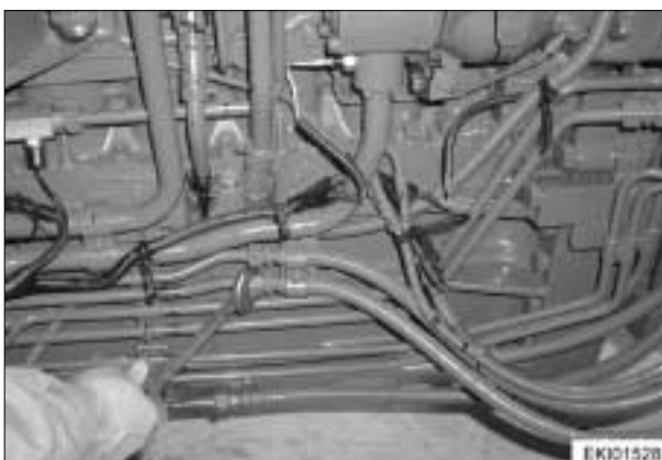
Fit hydraulic lines to steering cylinder.
