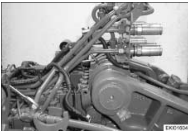
Fit hydraulic lines for EPC-DA switchover.
