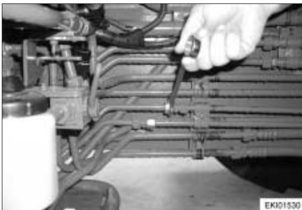
Fit hydraulic lines to front PTO.
