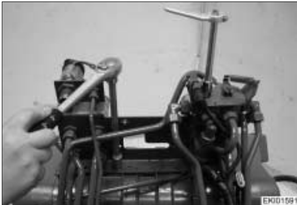
Fit bracket for hydraulic couplings.
