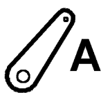
Fig. 4 Key on membrane keypad with "Active" LED on control console Rapid lowering system only available on rear power lift
