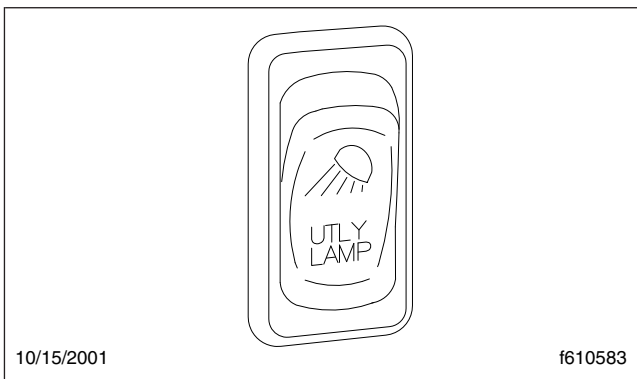
Fig. 5.10, Utility Light Switch
