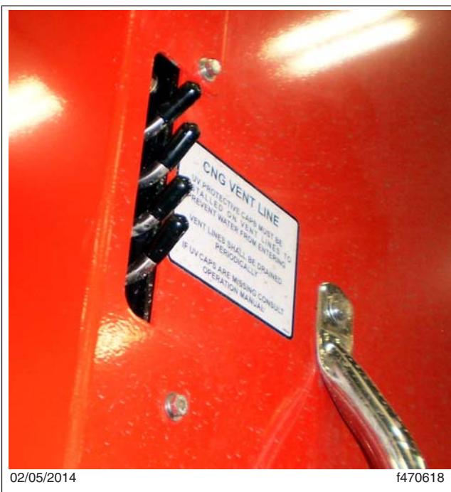
Fig. 21.8, CNG Vent Line Caps
