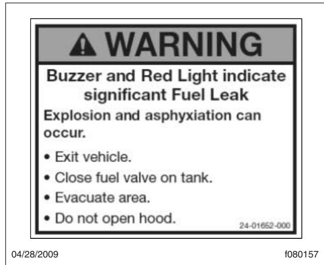
Fig. 25.4, Interior Warning Sticker
