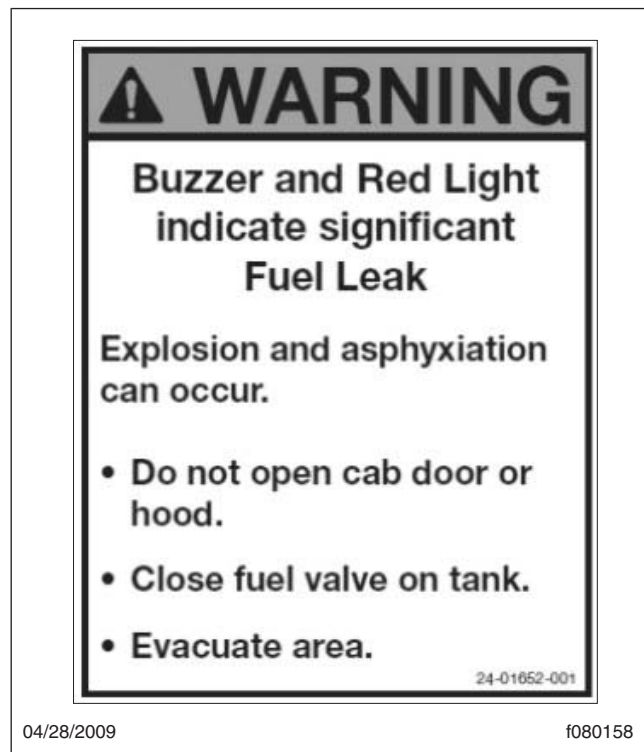
Fig. 25.5, Exterior Warning Sticker
