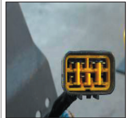
Stop and tail lamp side part number 897364-5310
