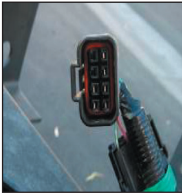
Chassis harness side part number 897364-5300
