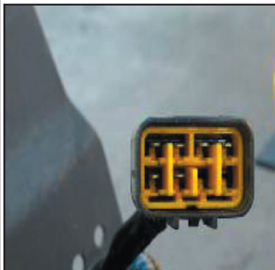
Stop and tail lamp side part number 897364-5310
