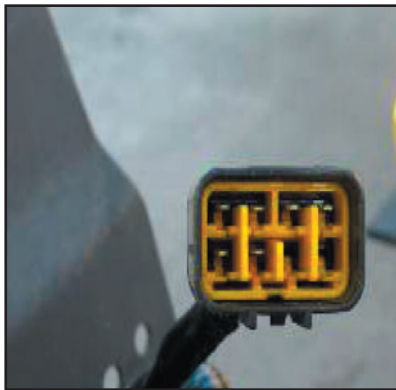
Stop and tail lamp side part number 897364-5310
