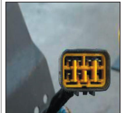
Stop and tail lamp side part number 897364-5310
