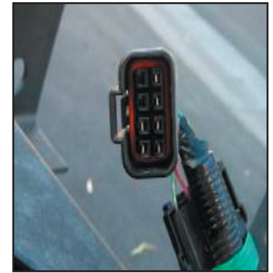
Chassis harness side part number 897364-5300
