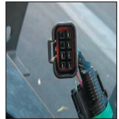
Chassis harness side part number 897364-5300
