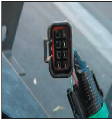
Chassis harness side part number 897364-5300
