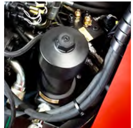
Improved placement of hydraulic filters.
