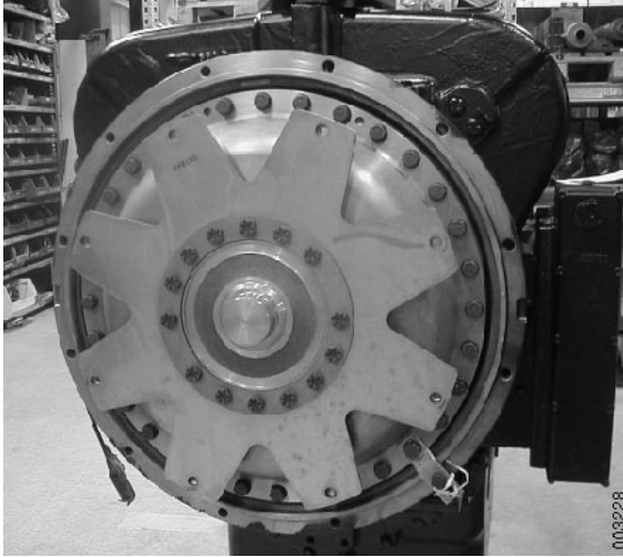
Attachment of flex plate.
