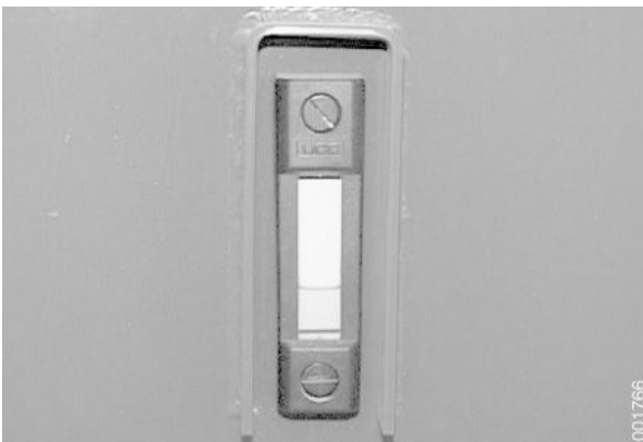
Relief valve for top lift, the figure shows an open valve.
