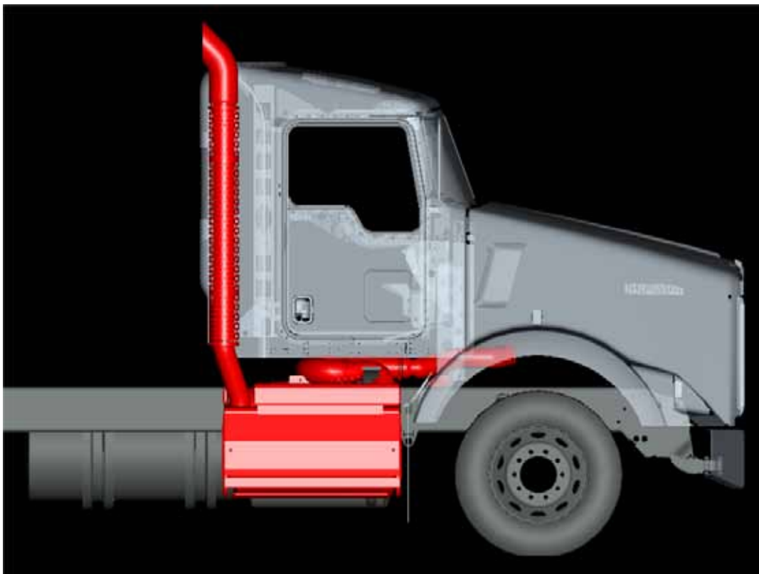
FIGURE 4-13: Right View of Right Hand Under DPF and SCR with Single SOC Tailpipe
