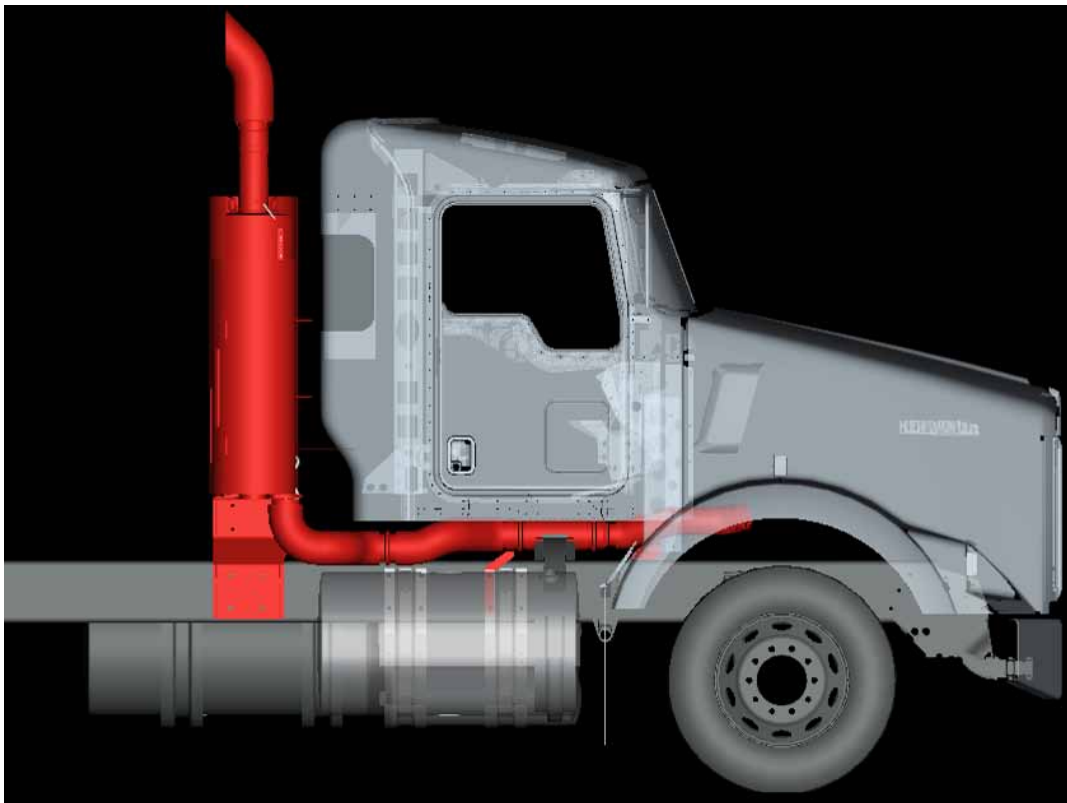
FIGURE 4-33: Right View of Vertical DPF and SCR
