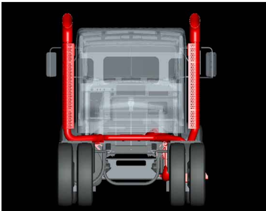
FIGURE 4-18: Back View of Right Hand Under DPF and SCR with Dual SOC Tailpipes
