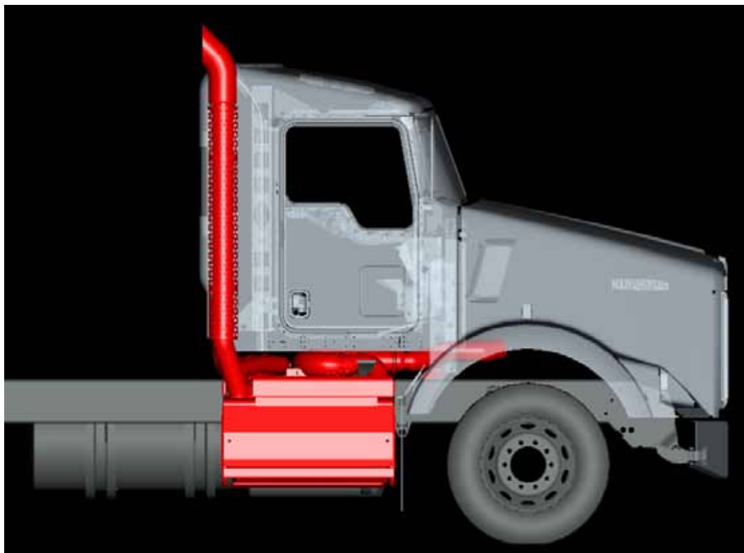
FIGURE 4-17: Right View of Right Hand Under DPF and SCR with Dual SOC Tailpipes
