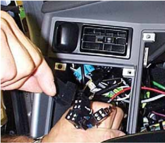
FIGURE 8-16. Spare Relay Connectors
