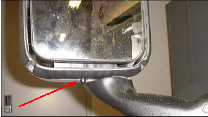
FIGURE 2-4: Aerodynamic Mirror OAT Sensor Location
