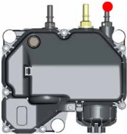
FIGURE 4-1: Measurement Location of DEF Supply Module (Pump)
