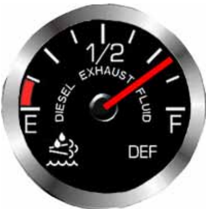
FIGURE 8-2. Diesel Exhaust Fluid Gauge
