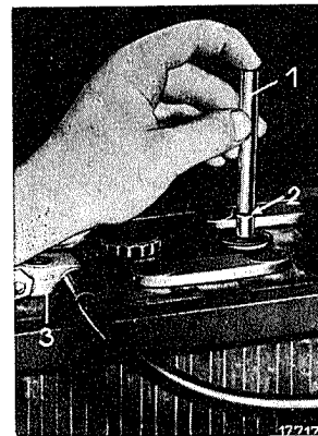
Picture 54-1/1 Check acid level
