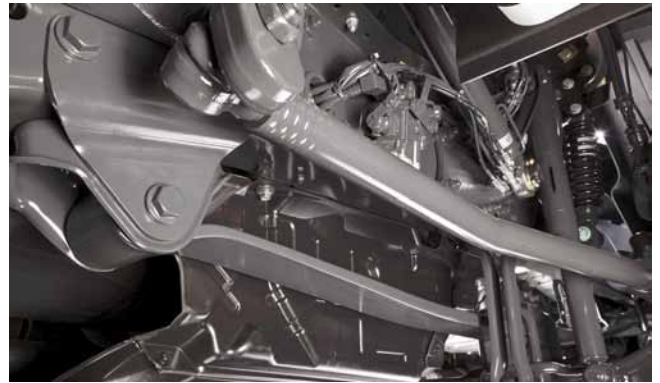
Front spring, 3.6 t, parabolic (Q1J)
