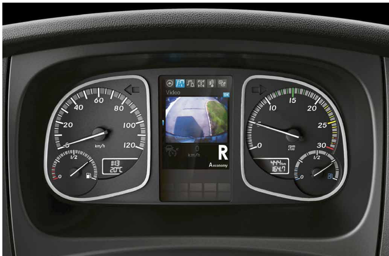
Instrument cluster 12.7 cm, with video function (J1C)
