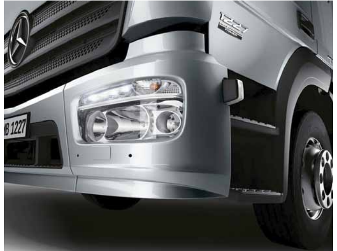
Halogen headlamp with LED daytime running lamps (L1C)
