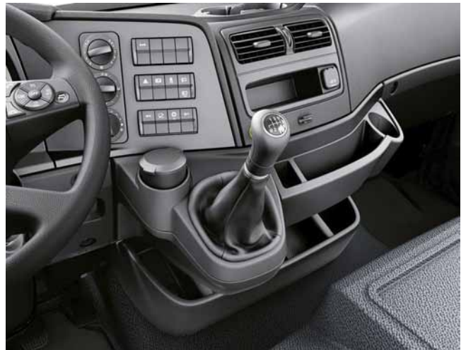
Shift-by-wire switching unit
