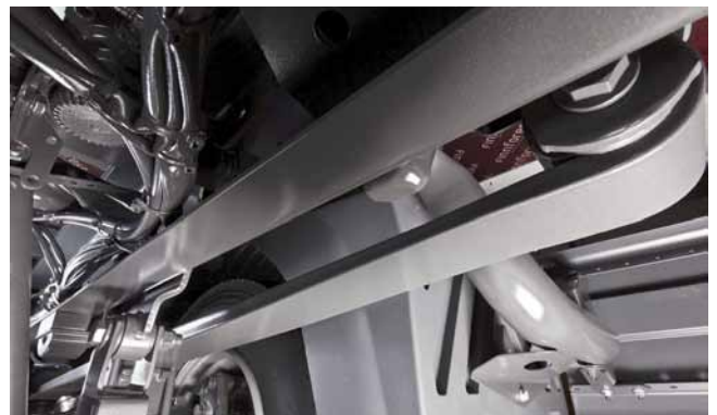
Rear spring, 5.0 t, parabolic, 1-leaf (Q2N)
