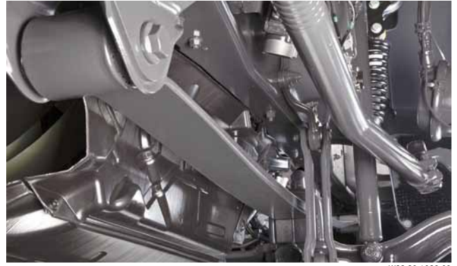
Front spring, 3.4 t, parabolic (Q1C)
