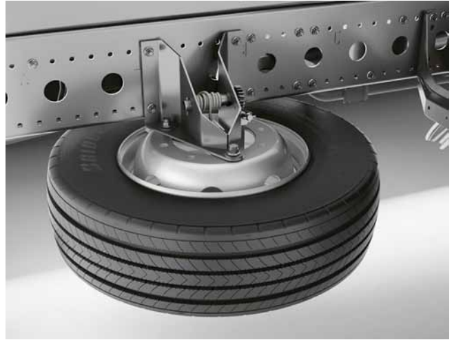
Spare wheel jack, on the side (R8A)
