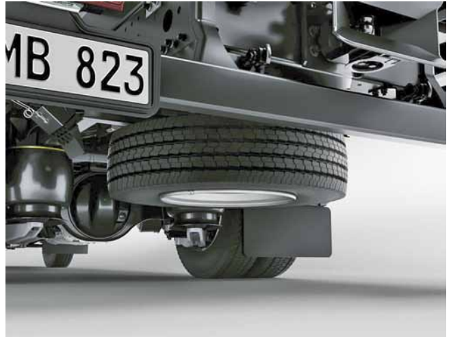
Spare wheel jack, behind the rear axle (R8D)
