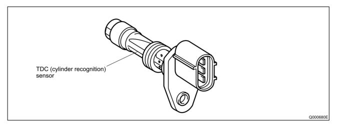
The No. 1 cylinder is located 78°CA from the No. 1 TDC reference signal following the irregular pulse. The interval between each cylinder is the same degree.
