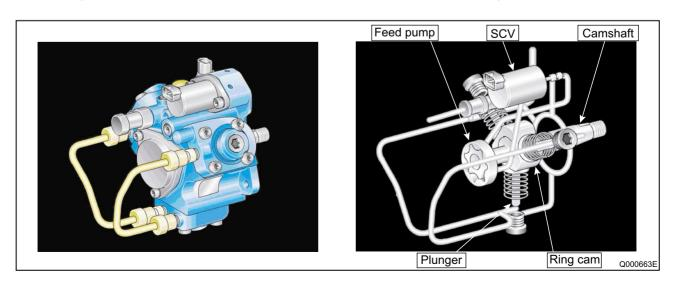
• As the camshaft makes one rotation, the positional relationship between the ring cam and the plunger remains unchanged. Each plunger makes a single reciprocal movement to pump the fuel. Fuel is drawn in by the feed pump, and the suction quantity is adjusted by the SCV (Suction Control Valve).
