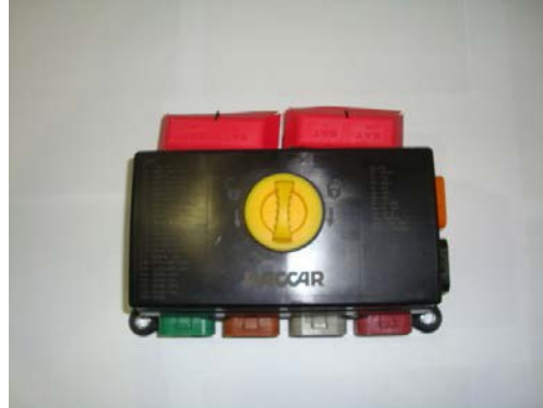
Figure 7.6.1 Pwer Distribution Center
