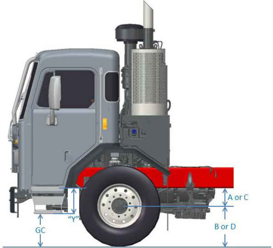
FIGURE 3-28. Ground Clearance Calculations
