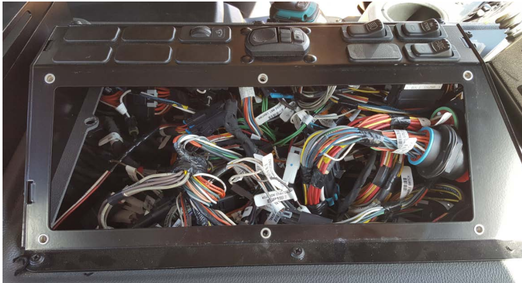
FIGURE 6-5. Body Builder Connections in Cab
