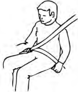
Incorrect (too high on hips)
