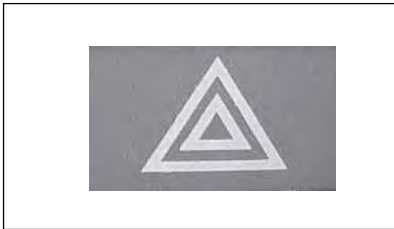
Hazard warning indicator
