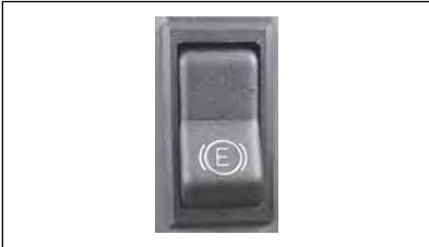
Exhaust brake isolator switch
