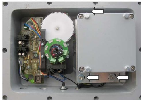
Angle sensor adjustment (see arrows above)
