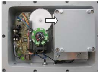
Length sensor adjustment (see arrow above)
