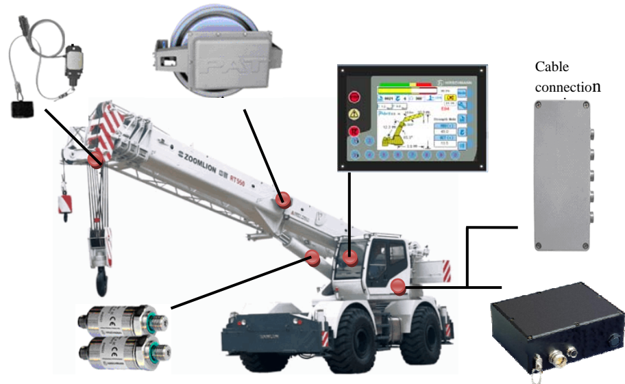
HC4900 LMI System configuration
